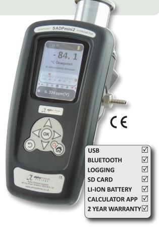
Connection to a pc via USB also enables the user to modify and save the set up and save details via the pc. The optional logging package adds Bluetooth® communication as well as very powerful logging and graphing capabilities. A cell phone app is available for communication with Bluetooth® cell phones and tablets.
